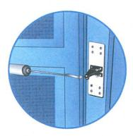
2 Mount Ultra Jamb Reinforcer™ universal screen door bracket to plate with four #10 roundhead machine screws.
